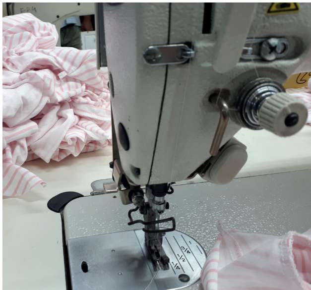
Follow up CAP protection installed on sewing machine
